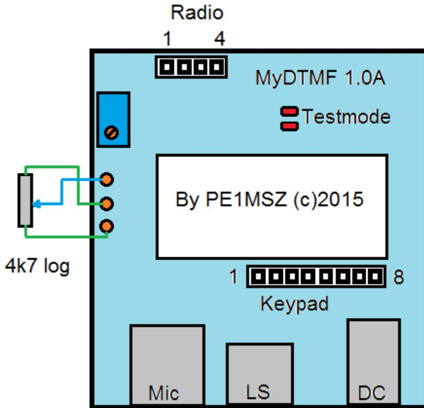
Image 1 : The board and it's connections.
